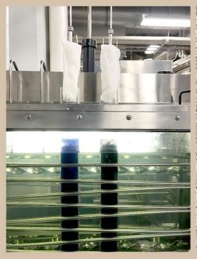
Machine used for samples: Ahiba Texomat
